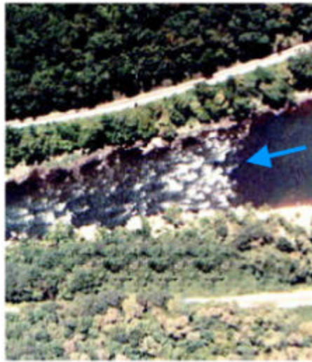
Figure 17: McCabes Rapid caused by partial reworking of debris-flow deposit on right valley wall resulting in the formation of a debris-bar deposit.
