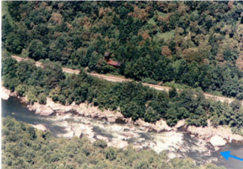
Figure 14: Double Z Rapid caused by large complex failure deposits on both sides of the stream channel.
