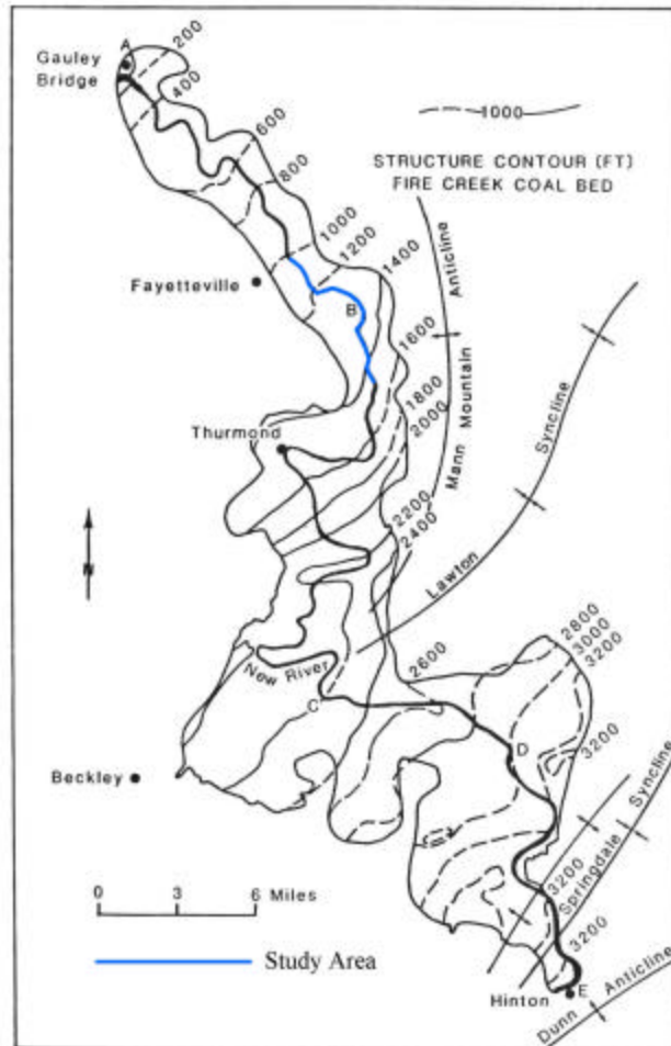
Figure 3: Structure contour map of New River Gorge based on the bottom of the Fire Creek Coal. (Modified from Englund and others, 1982)
