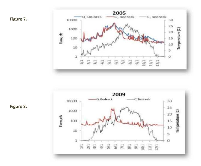
**Figures 7 and 8.** Thermographs and flows from contrasting spill years in 2005 and 2009. Ample flows in 2005 allowed for a gently tapered thermal response; in 2009 uncertainty regarding the volume and timing of runoff created thermal spikes and dips, which create poor spawning conditions for native fish.
