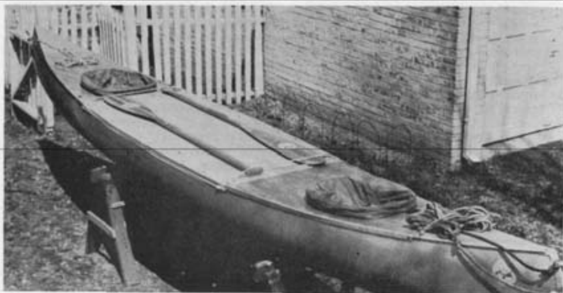
How the three-piece deck looks on an 18-ft. Grumman. Note spare paddles.
