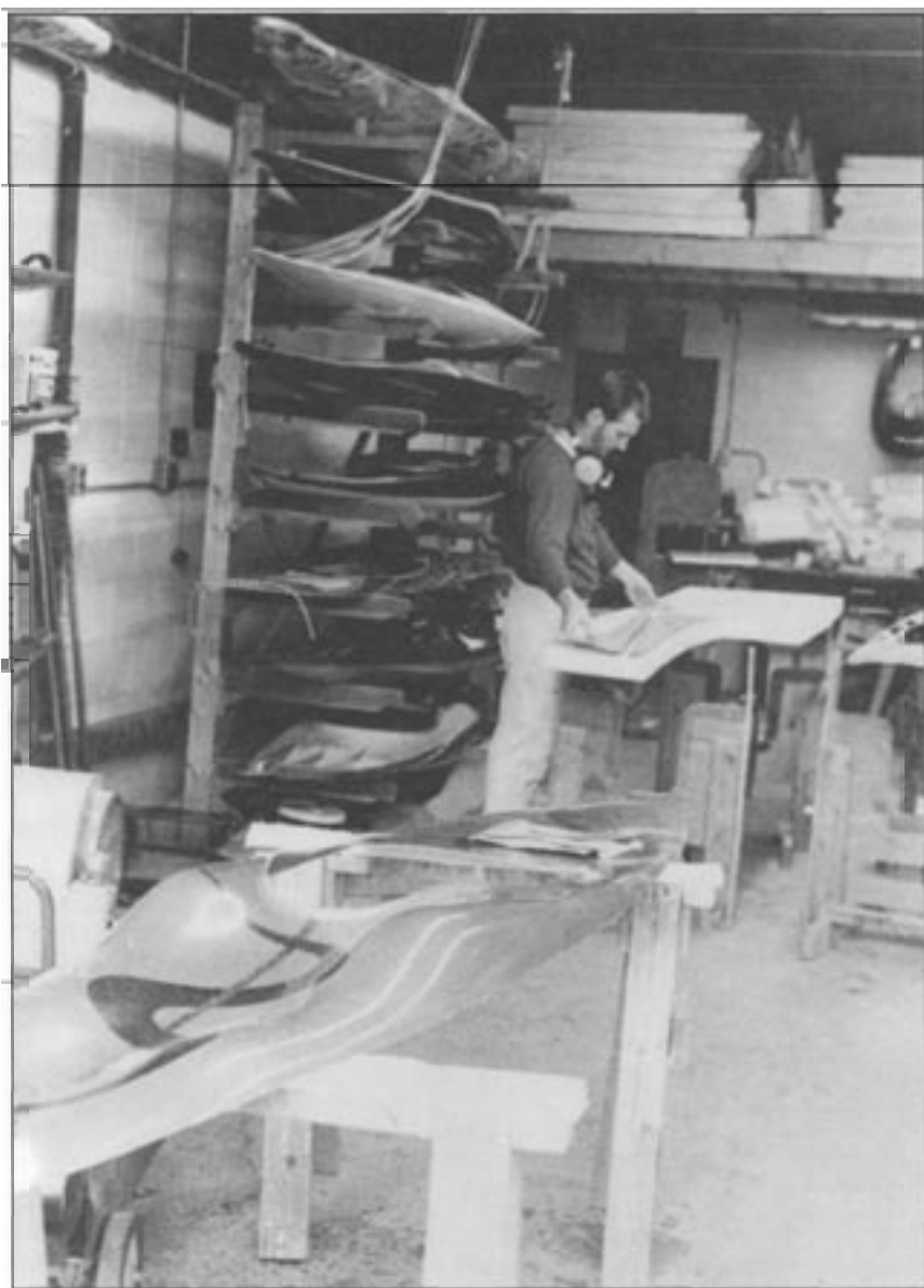
In the foreground of the New Wave workshop, a custom deck to a Vulcan awaits seaming while in the rear, foam pillars are cut for a low-volume kayak.
