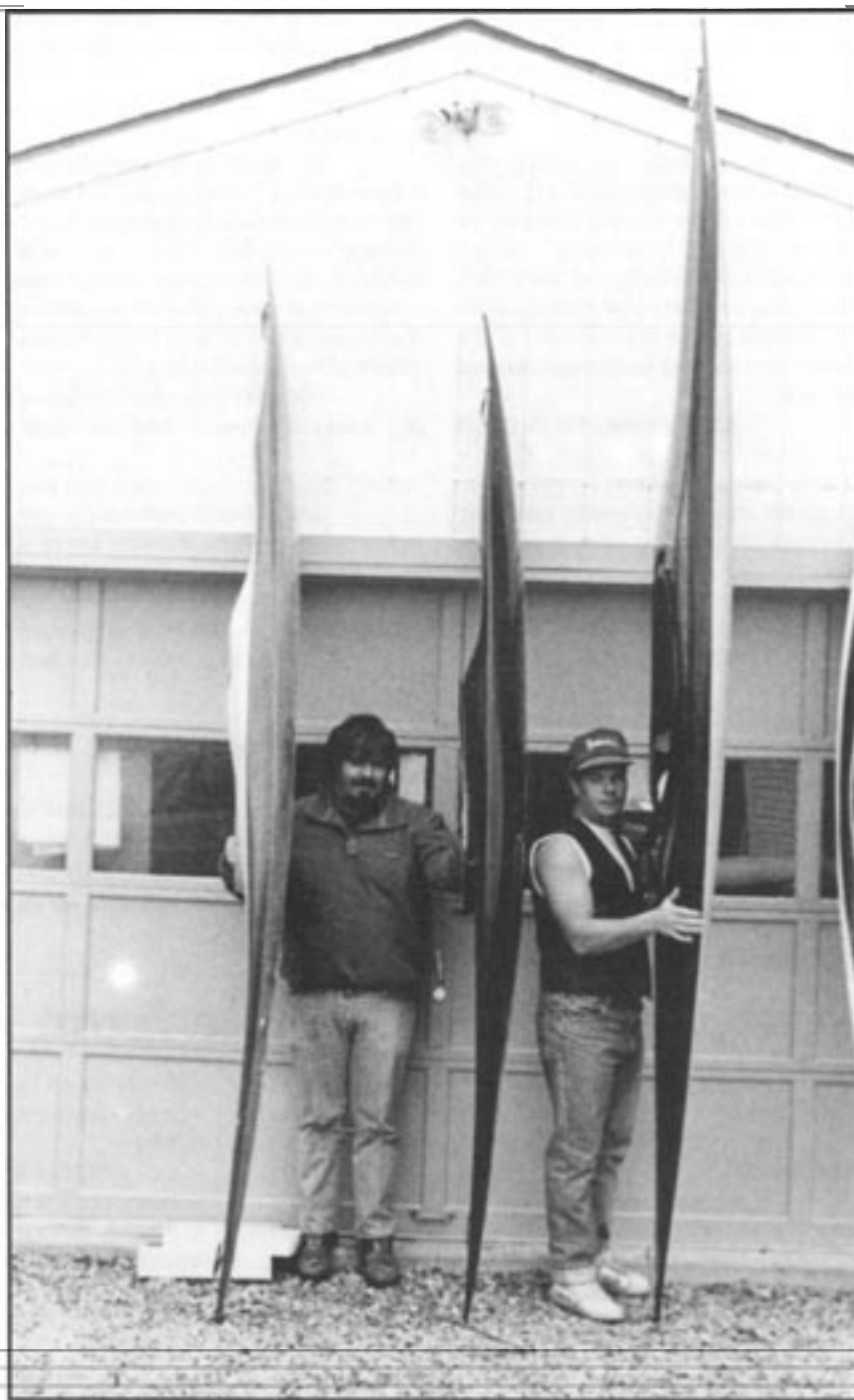
Basic design differences between squirt boats and cruising squirt boats are apparent in this comparison. Note the shorter length and harder long-axis rocker of the Vulcan and ProJet on the left. A closer inspection also reveals the rounded "floating hull" of the squirt boats while the Falcon (right) is built with hard rails.
