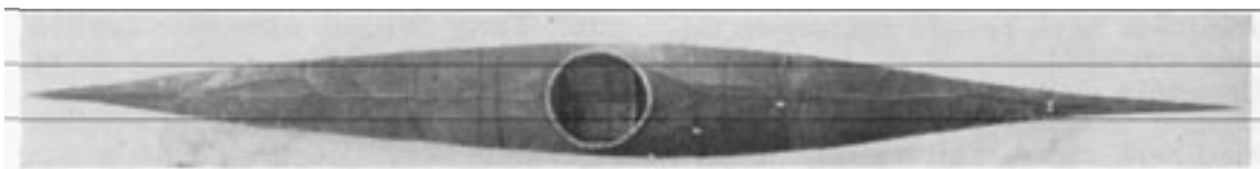
The same kayak seen in plan. Beam: 21 inches.
