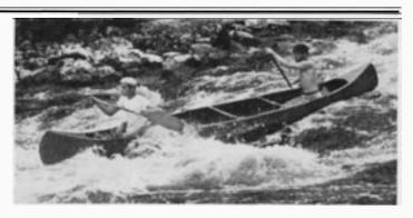
White water action demands quality! Only Grumman matches identical die-formed, heat-treated hull halves...rivets them close-spaced to an extruded keel...adds extra rigidity by bracing with wrought aluminum ribs, thwarts, and extruded gunwales. Plastic foam, fore and aft, provides positive flotation.
