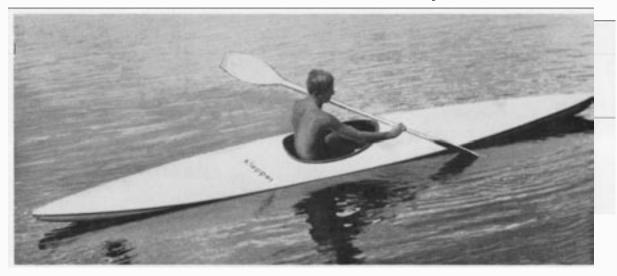
1: KLEPPER "QUIRL" — for White Water down-river . . . Weight: 44 lbs. (20 kg); length: 15 ft. (450 cm); widih: 25-1/5" (63 cm) . . . Comparable model: Klepper Folding "T-67". 2. KLEPPER "SL" While Water
