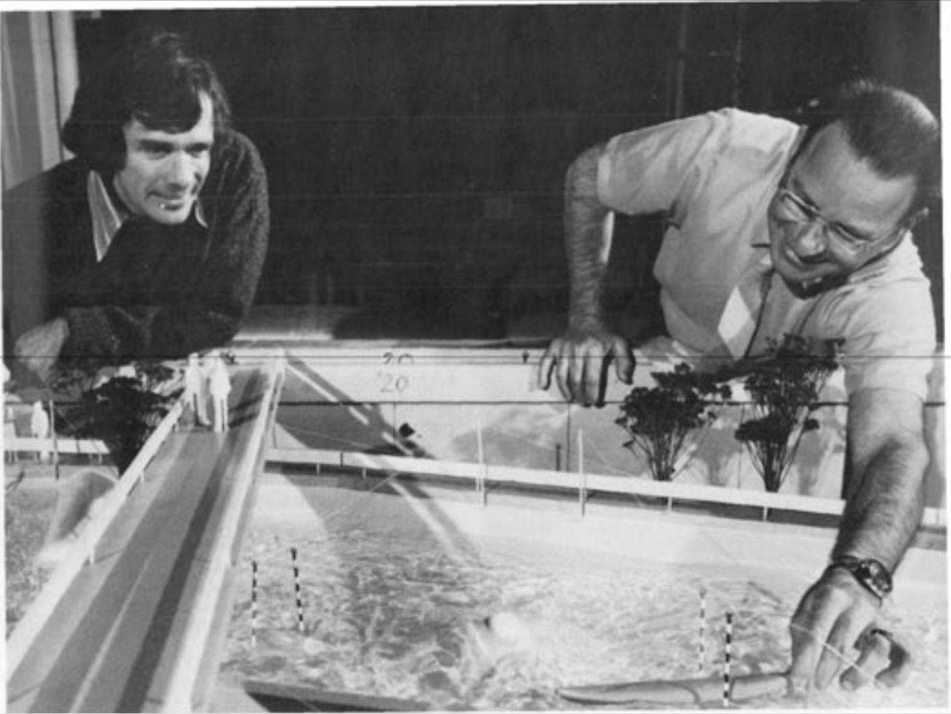
Ron Mason (left), originator of the whitewater park proposal, and Bill Simmons, a Reclamation hydraulic expert, send a hand-cawed model kayak down the chute. Bureau of Reclamation photo by R. A. Pauline.
